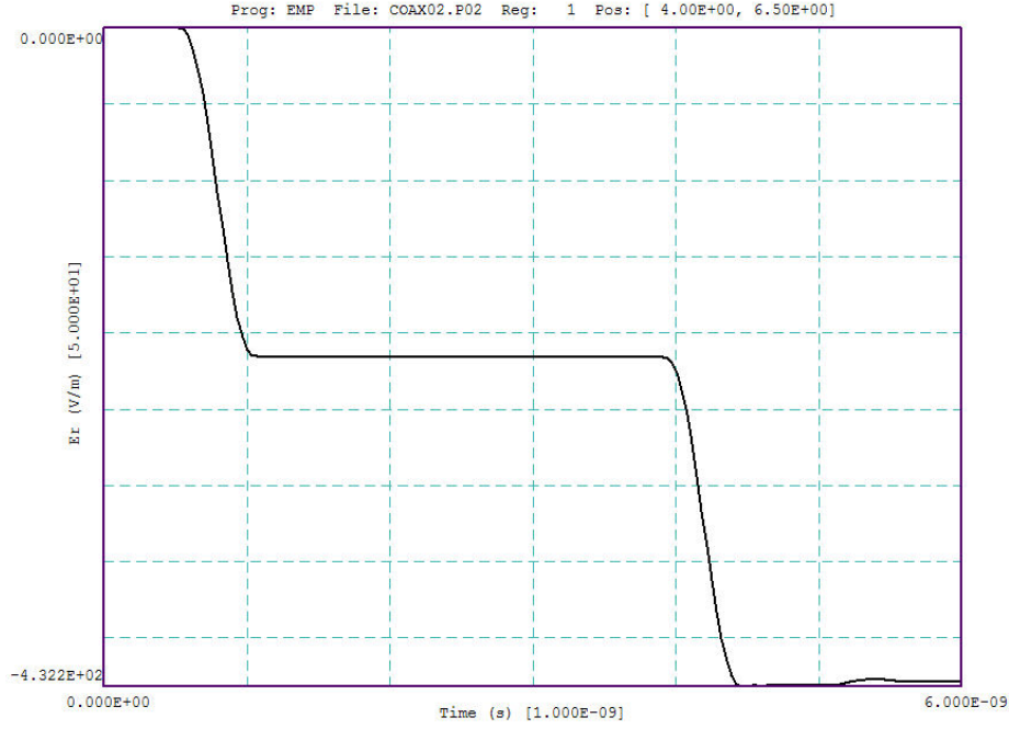
Figure 20: Example COAX02: temporal variation of E_r at position z = 4.0'' , r = 6.5'' .
