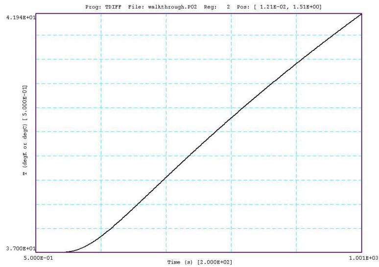
Figure 7: Plot of the time-variation of temperature at the probe position created by the Probe program.
